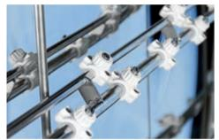
Dedicated washing and rinsing spray nozzles. The washing and rinsing/disinfection horizontal pipes are equipped with numerous nozzles. Thanks to the oscillating movement, they cover the entire internal surfaces of the washing chamber and wash items. The circuits are controlled by pressure switches.
