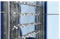
Multiple and separated horizontal washing and rinsing oscillating pipes grant excellent performance results.
